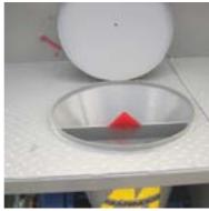
The use of a high shear venturi unit and the recirculation of the flow, guaranty homogeneous bentonite mixture.
